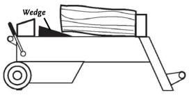
3. Repeat this process, using progressively larger Wedges, until the jammed log is free (*Figure 12*).
